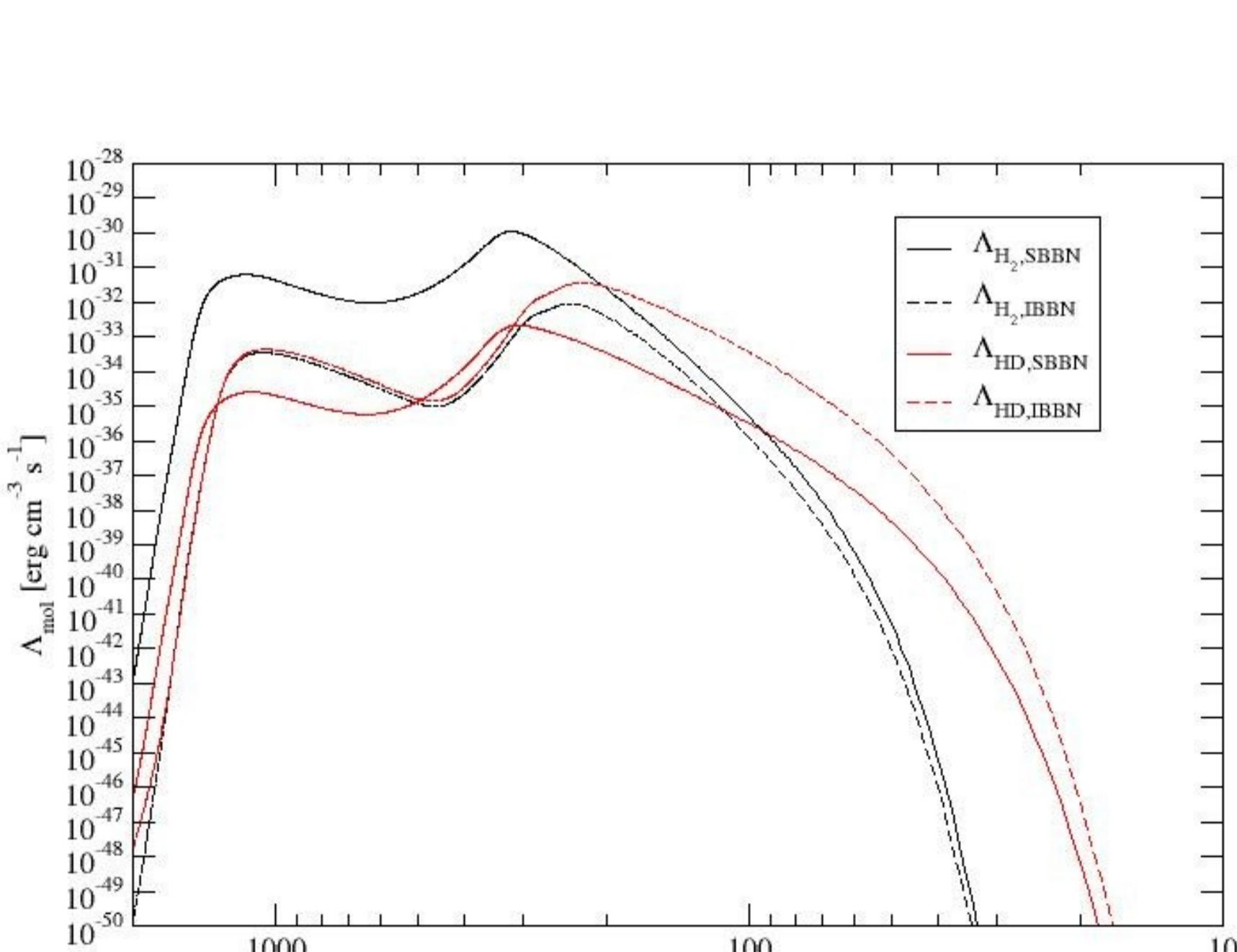
H<sub>2</sub> and HD cooling functions in both scenarios. SBBN:  $\Psi_{\text{HD}}$  dominates for redshifts smaller than about 90. Non-homogeneous model:  $\Psi_{\text{HD}}$  is always greater than  $\Psi_{\text{H}_2}$ .
