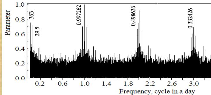
Deeming amplitude spectrum and spectrum of window
