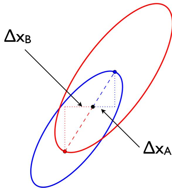
$$\text{mass ratio } q = M_B / M_A = \Delta x_A / \Delta x_B$$
